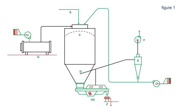
As described before, in this type of chamber the drying process is Split in 2 stages. The first stage happens in the proper drying chamber and the second in the fluid bed dryer that gathers the powder exiting the chamber. This fluid bed receives a hot air current that has two functions: fluidizing the product and finish the drying process (2nd stage)
